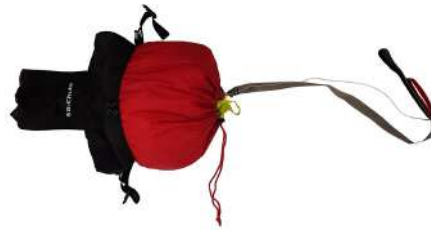
Make sure that there is only a little of the riser visible, while the rest is stored in the red pocket. Close it with the rope.
